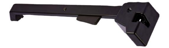
The compact 050-7120 10mm Single Rotor Latch with Handrail is designed for operator and compartment door applications for off-highway vehicles that require a remote interior release. The latch is incorporated into a rectangular tube for support for the opening and closing function of the door and provides for greater ease of operation (ergonomics) over direct releases.
